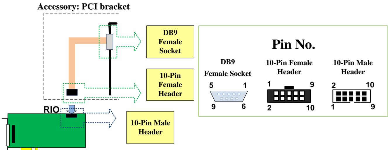
Fig. 3-9 Description of the PCI bracket
