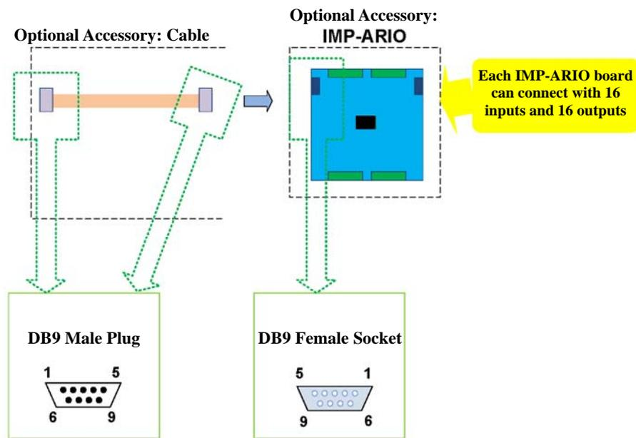
**Fig.3-10 Description of the cable and the connector on the IMP-ARIO**
