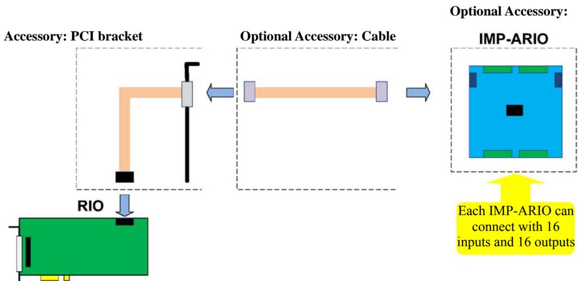
Fig. 3-8 Diagram of the connection between the IMP-2 and IMP-ARIO
