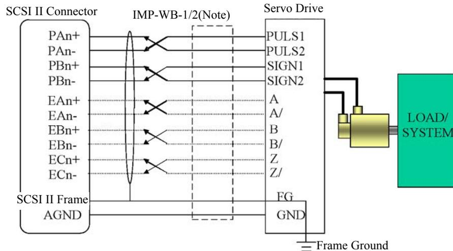
Note: This figure is an example for any axis of the IMP-2. Use the same diagram for other axis (where  $n=0\sim7$ )
