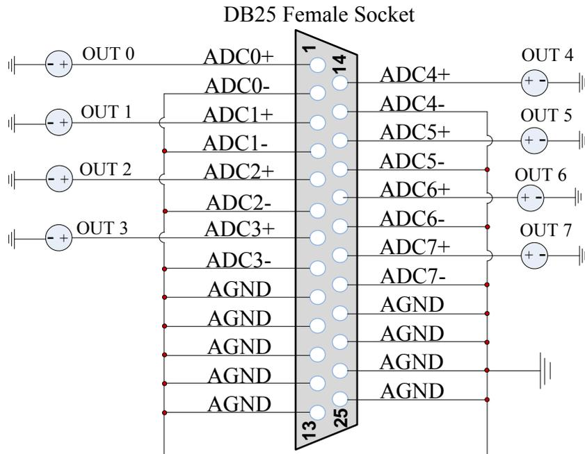
**Fig.3-12 Wiring of Single Ended Input**
