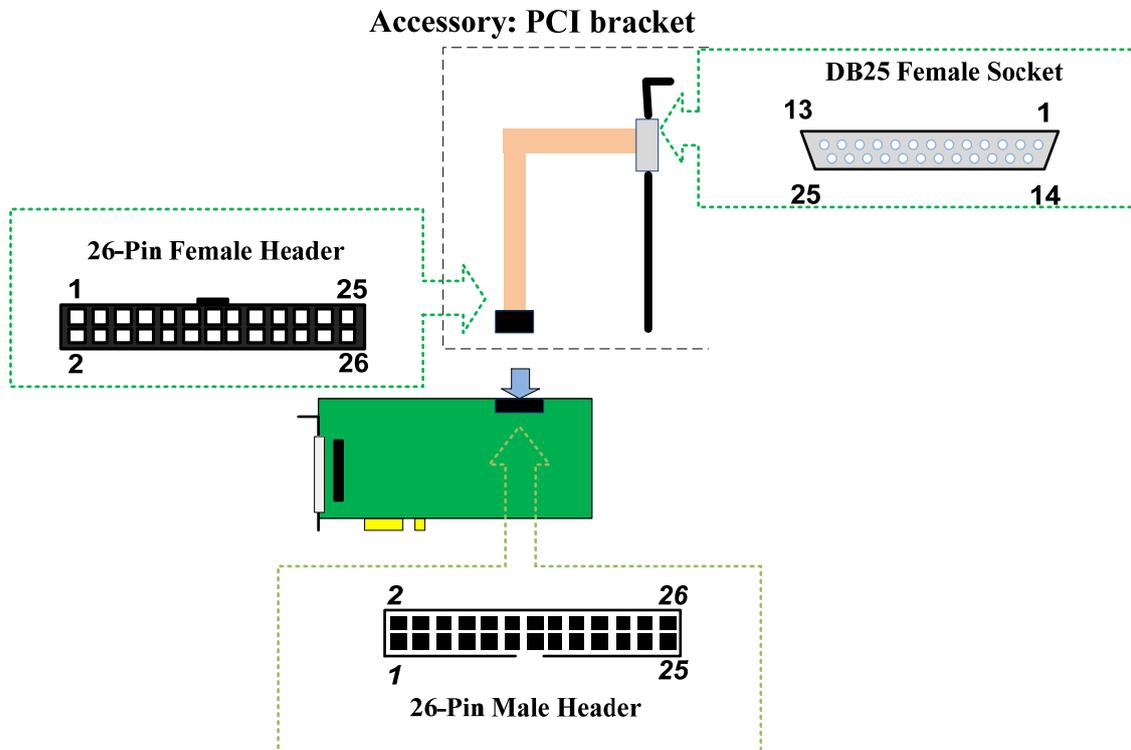
**Fig. 3-11 Descriptions of the ADC connector on the IMP-2**
