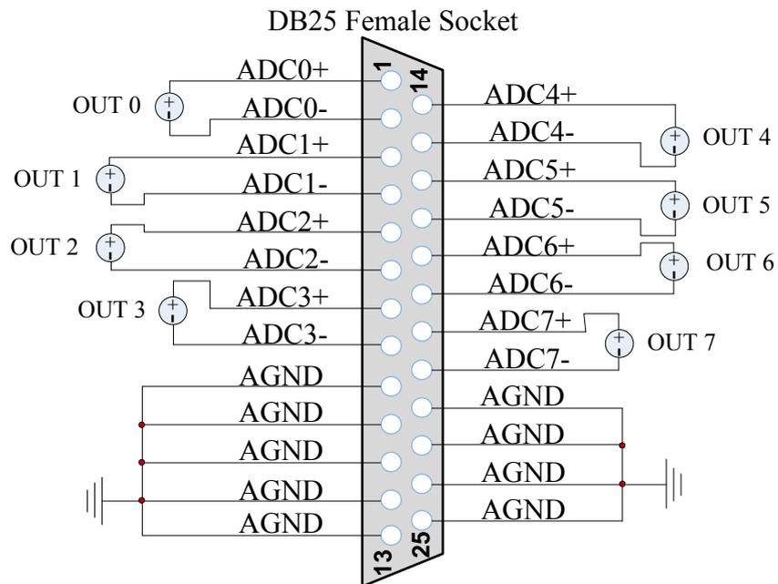
**Fig.3-13 Wiring of the Differential Input**
